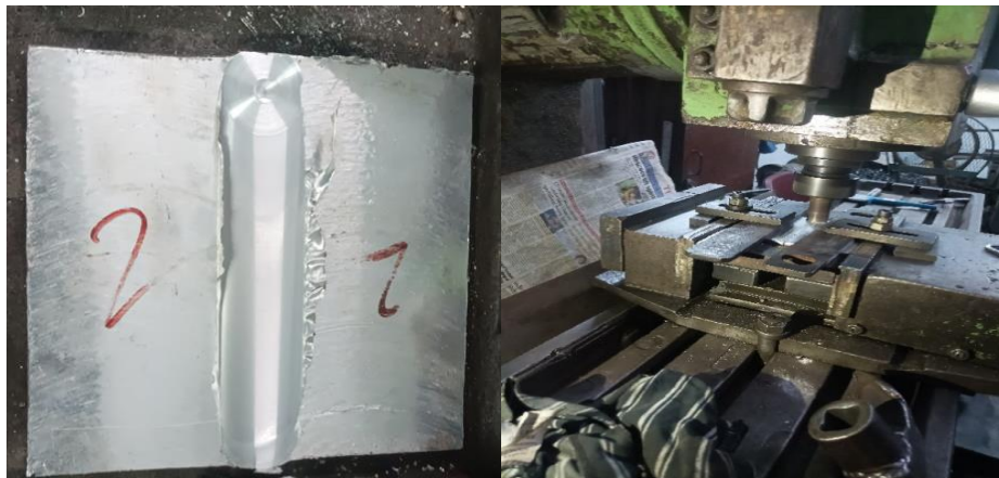
Fig:5 Final AMC joint Fig:6 Arrangement for experimentation
