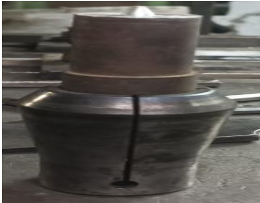
Fig:3 straight tapered cylindrical tool used for experiment
