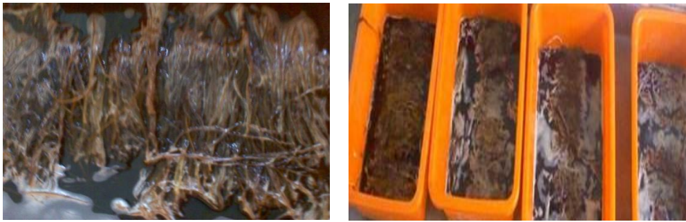
Fig 1: During pretreatment with 2,5,7,10 %NaOH
