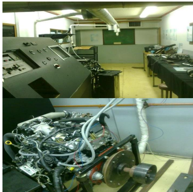
Figure 2: Engine Test cell facilities and IC Engines at UKZN for Moringa biodiesel experimentation
