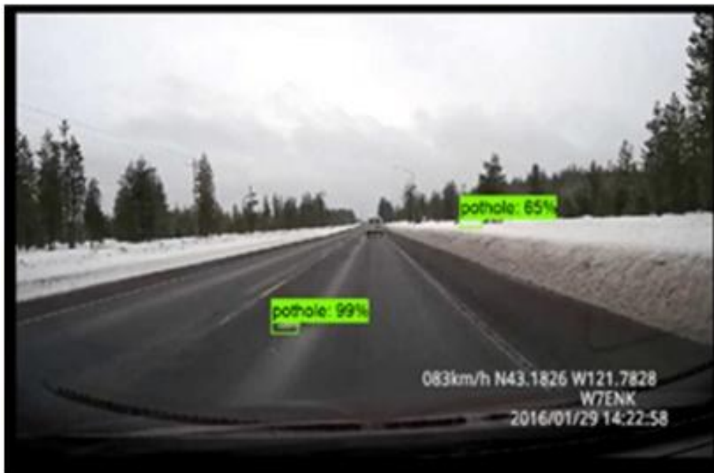
Figure 3. Detection of potholes using Camera [28]
