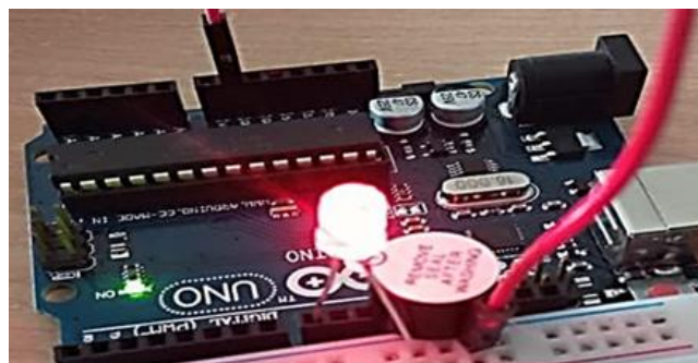
Fig. 10 The Buzzer and LED Turned on
