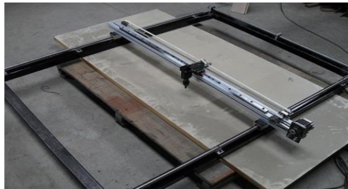
Fig 9: Final Assembly of Portable 3-Axis Cutting Machine Powered by Laser
