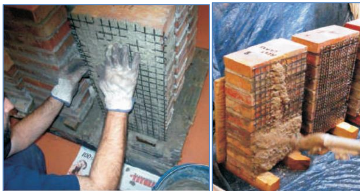
Fig. 3 The use of TRM to upgrade masonry [30]
