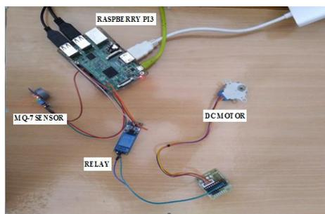
Figure 5: CO monitoring and control in vehicle by using Raspberry pi-3 system
