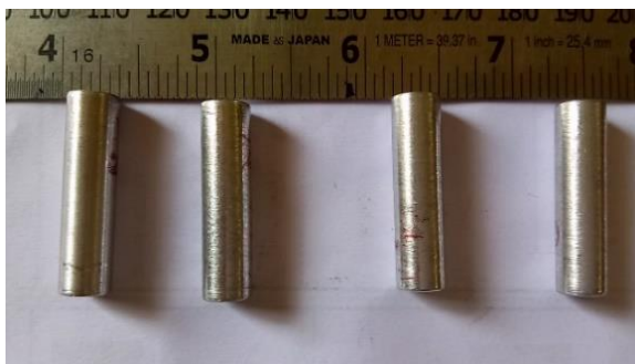
Fig1. Wear test samples: (a) 0% reinforcement, (b) 2% reinforcement, (c) 4% reinforcement, and (d) 6% reinforcement.
