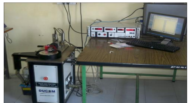
Fig2. Pin-on-Disc wear testing apparatus (Courtesy: R & D Centre, BIT, Bangalore)
