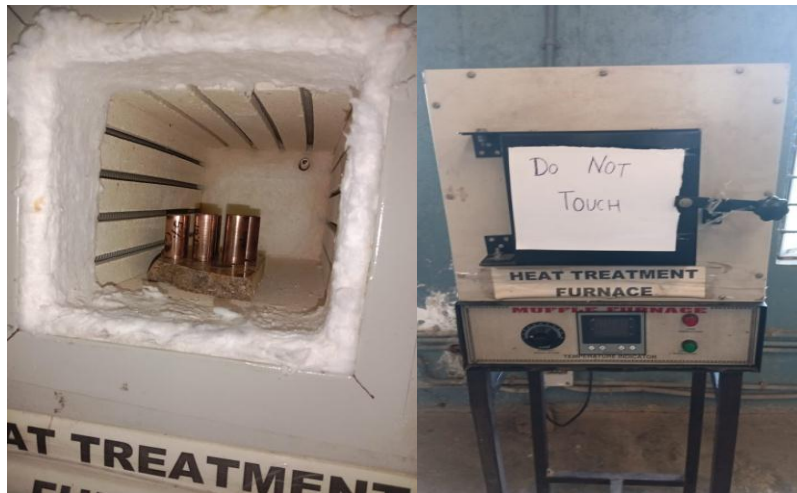
Figure 3: Experimental set-up for the sintering process
