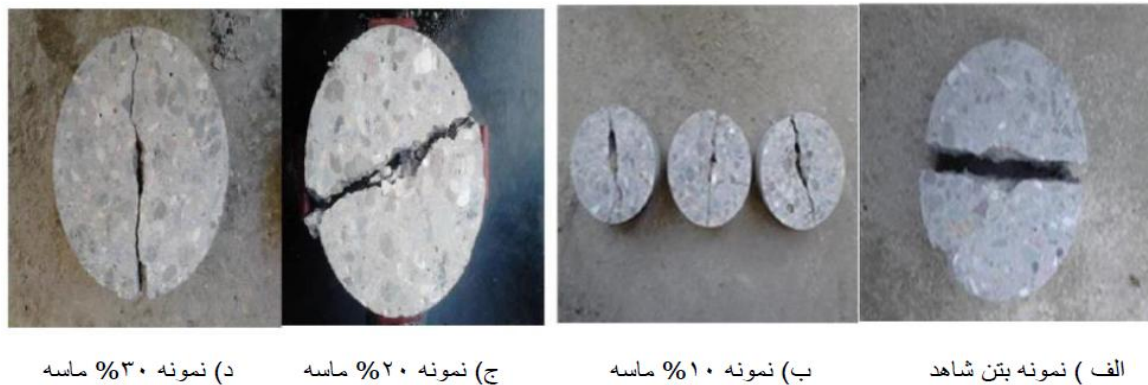
Figure 11: Waste concrete samples in different percentages of replacing bricks with fine grains a) control concrete b) 10%, b) 20% and c) 30%
