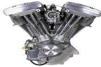
Figure 1: Air cooling system
