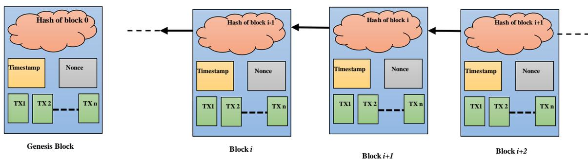
**Figure 1** Block chain data hashing method
