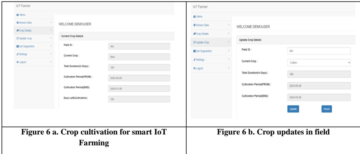
The field ID of a specific field is shown in figure 6 a) above, together with the crop that is currently being cultivated there and the total Day count for the crop will full growth. The beginning and ending times of a certain crop's cultivation as well as the number of days left in cultivation figure 6 b) represent the crop updates of that particular field.
