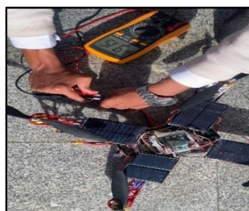
Fig. 3: Drone with solar cells
