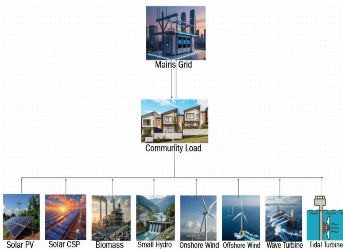
Fig. 3.4: Bottom-up hybrid mini-grid in interconnected mode
