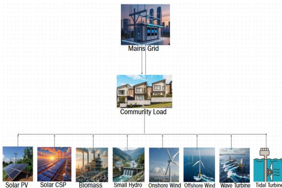
Figure 4.4: schematic of bottom-up renewable energy mini-grid including small hydropower
