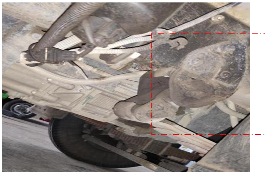
Figure 5. In-vehicle assembly configuration of the leaf spring mounting bracket, showing the spatial relationship between the bracket, chassis frame, and leaf spring assembly.
