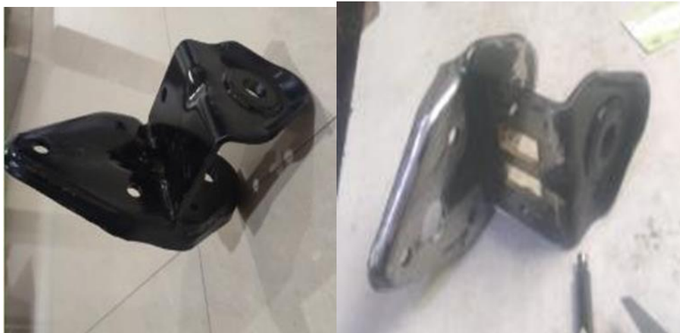
Figure 32. Visual comparison: (a) original leaf spring bracket, (b) topology-optimised bracket with rectangular horizontal slot and circular vertical cut-out. The two geometric modifications are clearly visible.
