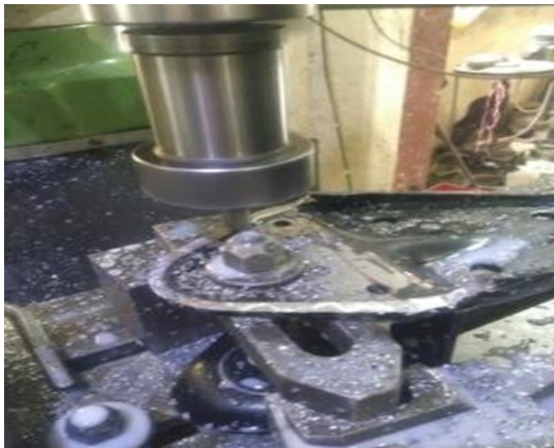
Figure 24. Circular cut-out produced by two-stage drilling (pilot hole followed by finish bore) on the vertical triangular plate.
