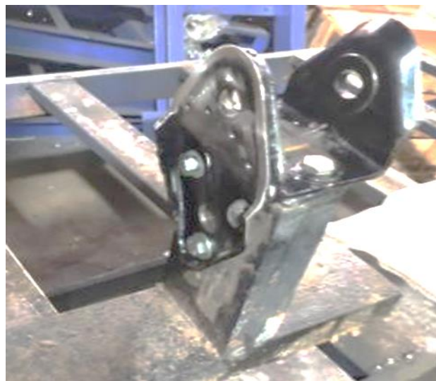
Figure 26. Optimised bracket assembled on the fabricated C-channel test fixture, secured with five high-strength bolts at the chassis attachment positions.
