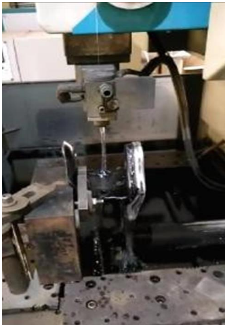
Figure 22. (a) Wire-cut EDM operation on the bracket horizontal plate. (b) Resulting rectangular slot produced to the required dimensional tolerance.
