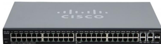
Figure 4. A Cisco switch
