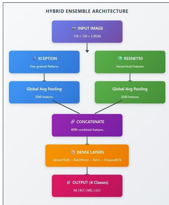
Fig. 2. Proposed Hybrid Ensemble Architecture Integrating Xception and ResNet50 for Skin Cancer Classification.
