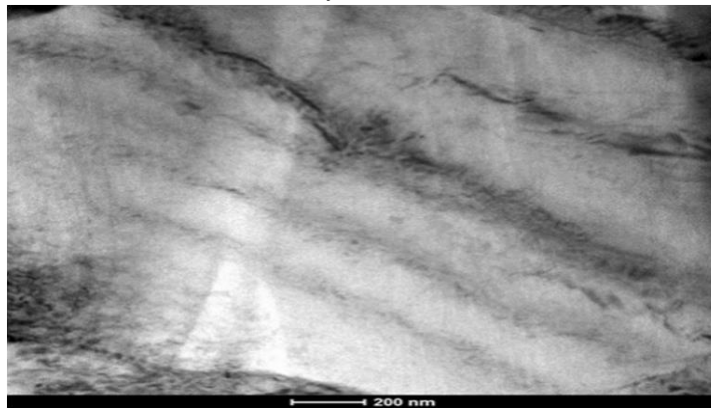
Figure 8: TEM microscopic image of 4% SiC reinforcement and particulate matrix reinforcement interfacial zone
