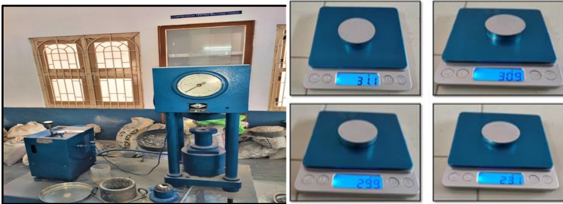
Figure 2: (a) Computerised compaction machine (b) AZ31D magnesium FGM specimens with reinforcements
