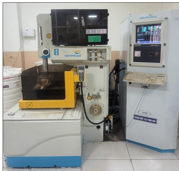
Figure 1. Electronica ELPULS 40A DLX Sprint-cut CNC WEDM machine
