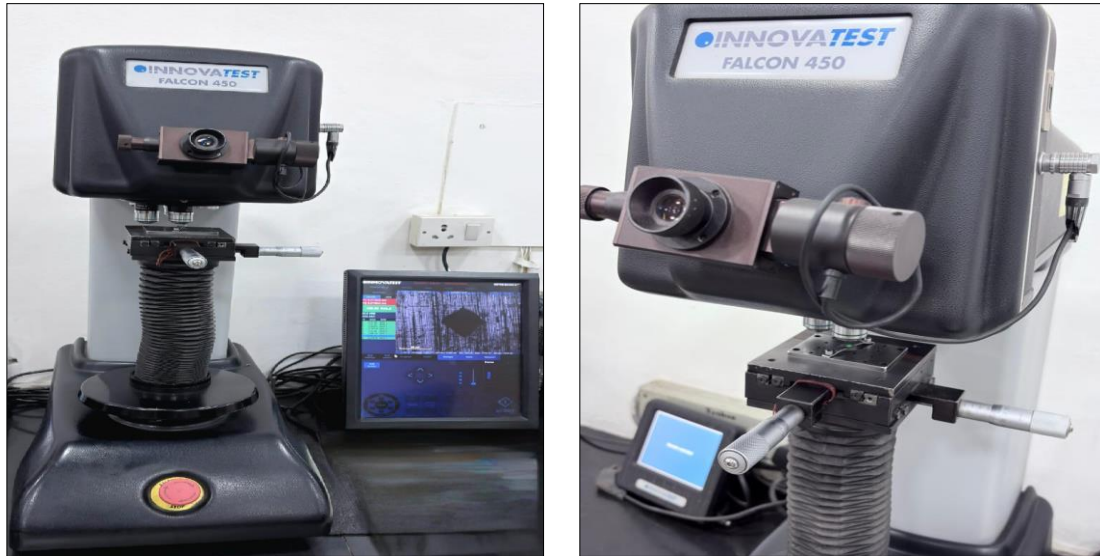
Figure 3. Vickers micro-hardness tester and sample mounted
