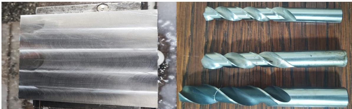
Fig 1: SS 410 Workpiece Material and M2 drills
