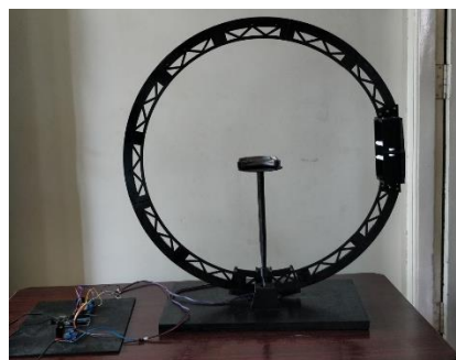
Figure: Final assembly of automated photogrammetry rig
