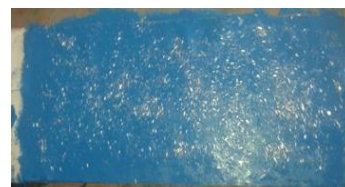
Fig 8: Sprinkling of Glass Flakes
