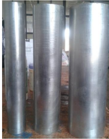
Fig 1: SS Pipes of Different Diameters for fabrication of shells
