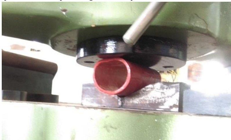
Fig 10: Lateral Compression of the GFRP Specimen
