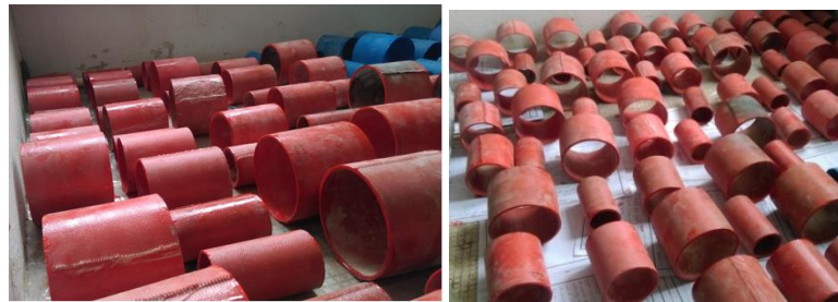
Fig 9: Edge Sealed GFRP composite pipes
