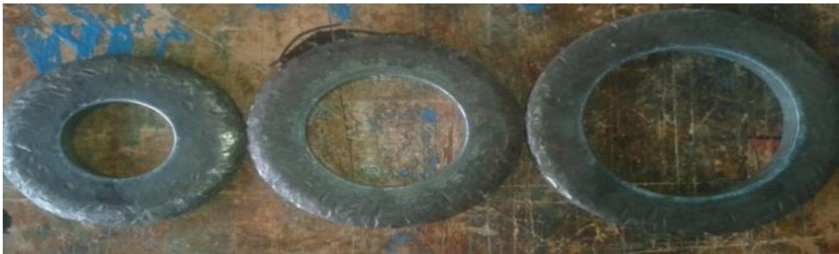
Fig 2: Extraction Fixtures for Different Diameters of shells
