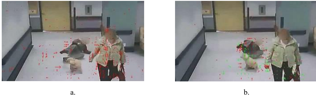
Figure 2: Sample video frames: (a) MPEG-4 (motion vectors in red (for P)), (b) H.264 (motion vectors in red (for P) and green (for B)).
