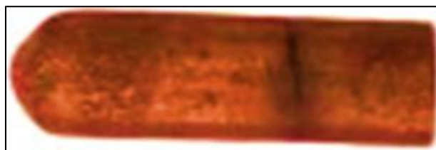
Figure 2: Copper-Coated Wear Test Specimens
