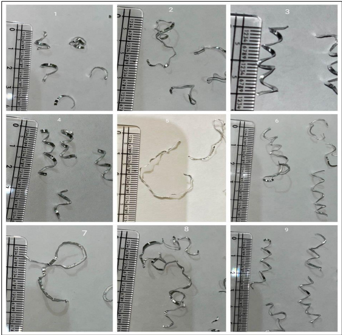
Fig. 5. Chip formation during experiments at different parametric settings.
