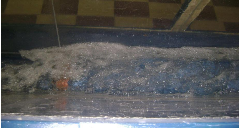
Figure 7. The jet phenomenon at the upstream toe of the jump (View from upstream).
