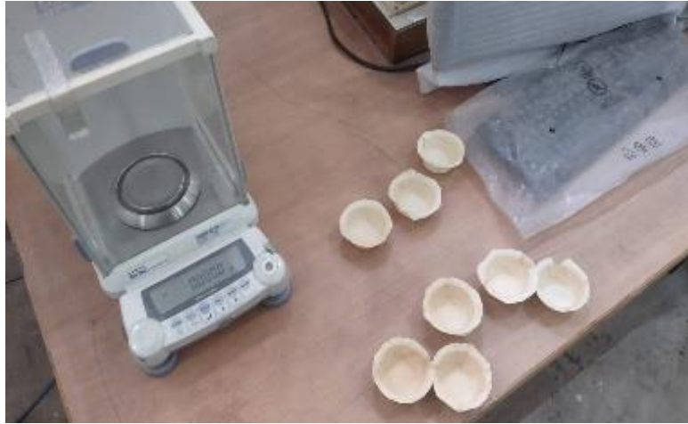
Fig.3.1. Dry weight and wet weight of corn husk cup being measured.
