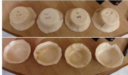
Fig 2.1. Corn husk heat pressed at different temperatures. (From left) 115, 120, 110, 100 degrees Celsius.
