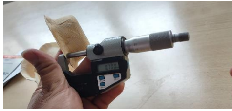
Fig.4.2.: Thickness of sample edge measured. (0.700mm)
